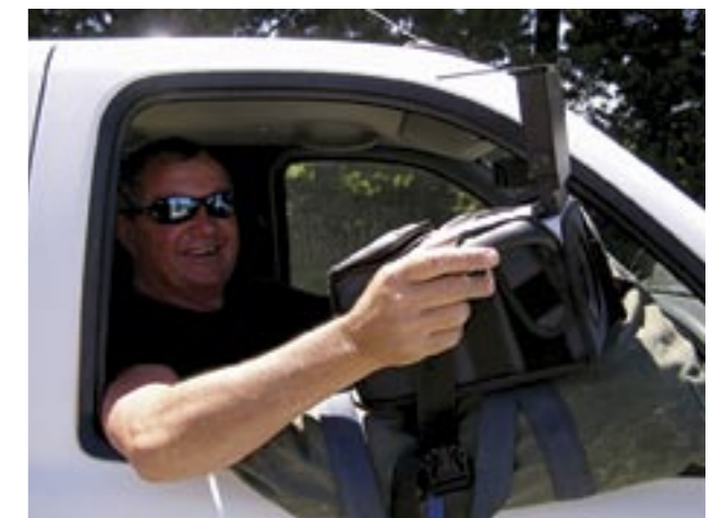
Above: Corona camera detecting faulty insulators on a rural line. The corona camera identifies defective equipment on our network that cannot be picked up by the naked eye or other commonly used maintenance techniques.
