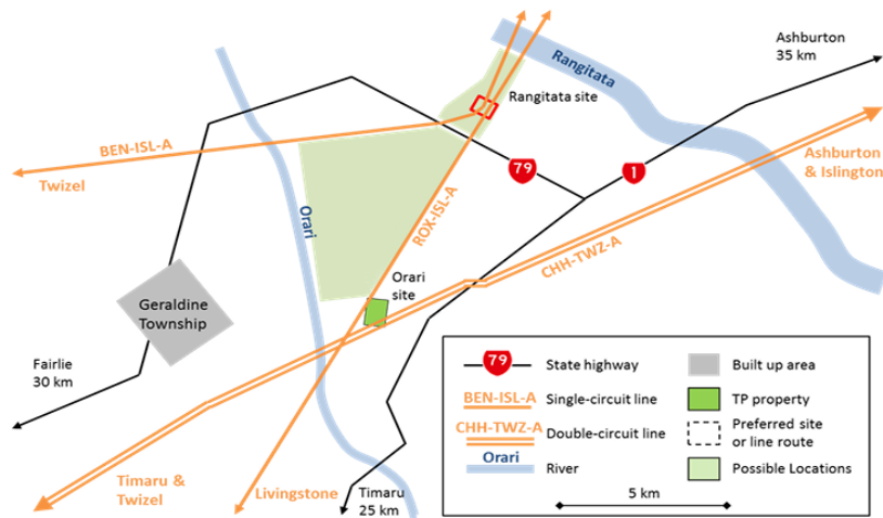
Figure 3.4: Potential Orari and Rangitata switching station locations
