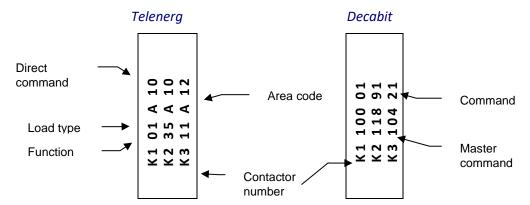
Both labels are examples of ripple relays that support a day/night retail tariff, where contactor 2 switches a dual register meter, contactor 3 switches the water cylinder on at night, and contactor 1 provides peak interruption to the customer's water heating override switch.
